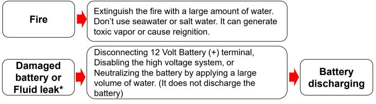
\*If electrolyte solution leakage, or any damage to the High-Voltage battery casing is observed.
