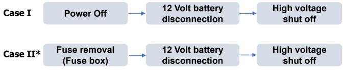
\*In case of the vehicle cannot be disabled using the "power" button.
