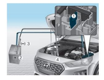
7. Connect the other end of the second jumper cable to the black, negative (-) chassis ground of your vehicle (4). Do not allow the jumper cables to contact anything except the correct battery or jumper terminals or the correct ground. Do not lean over the battery when making connections.
